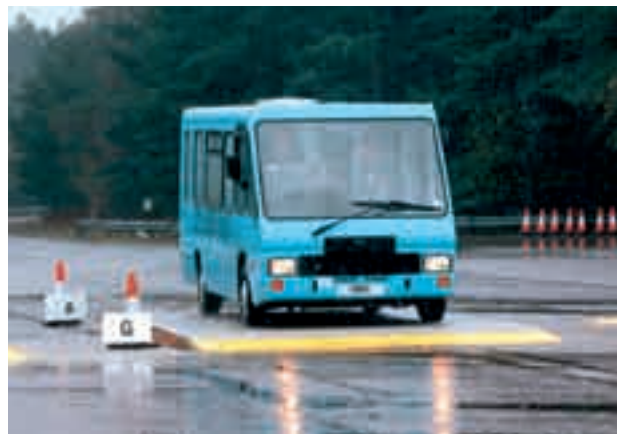
Fig. 2.1 Bus trials over flat-top humps
