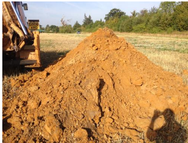
Photo 4: Arisings from trial pit TP02.
