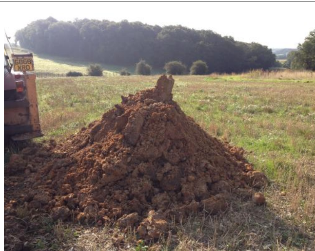
Photo 20: Arisings from trial pit TP08.
