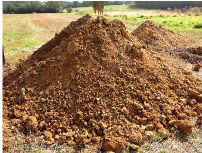
Photo 18: Arisings from trial pit TP07A.
