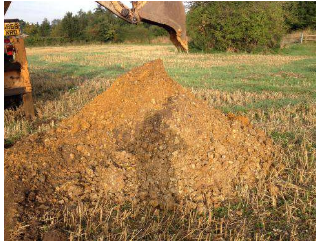
Photo 2: Arisings from trial pit TP01.
