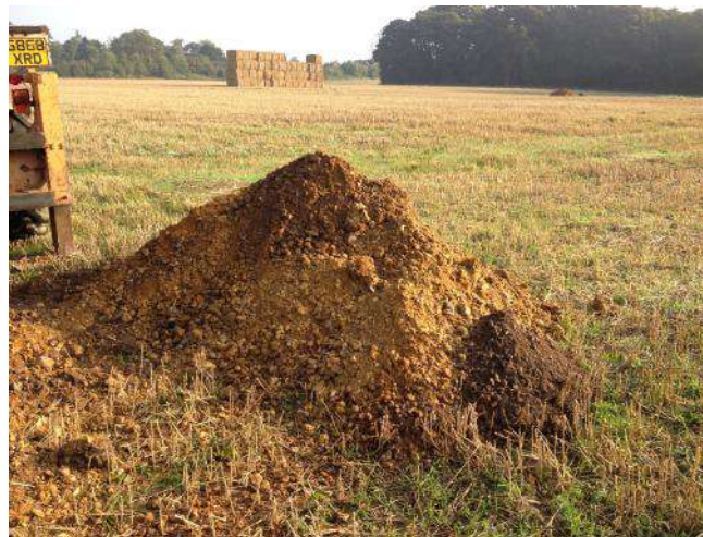
Photo 16: Arisings from trial pit TP07.
