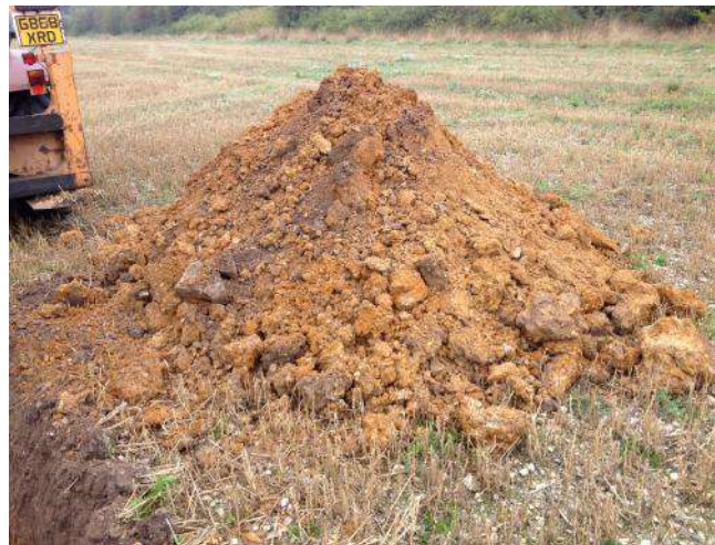
Photo 8: Arisings from trial pit TP04.
