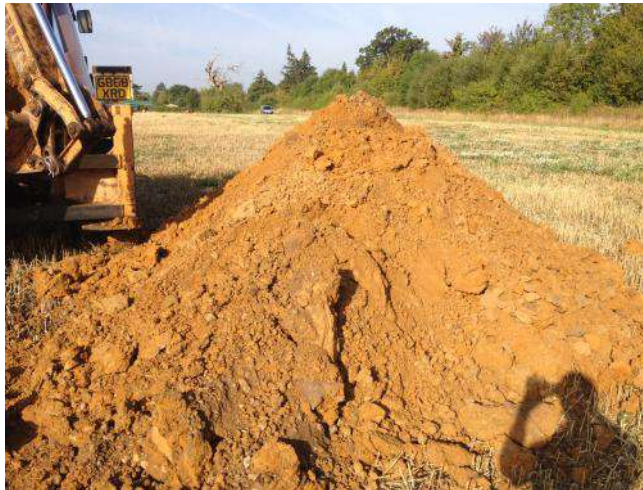
Photo 34: Arisings from trial pit TP15.
