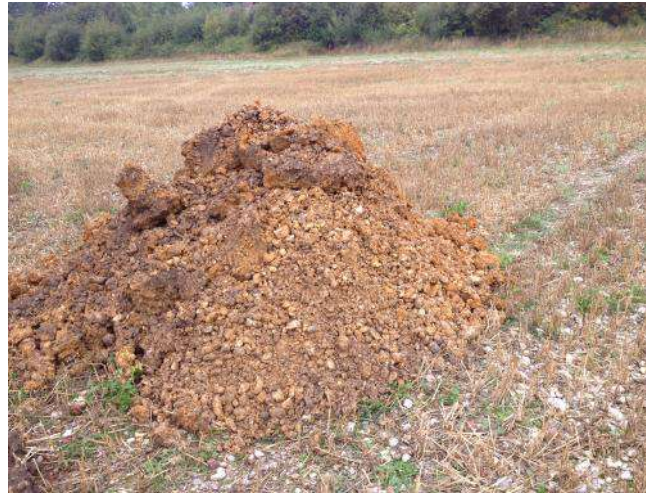
Photo 6: Arisings from trial pit TP03.
