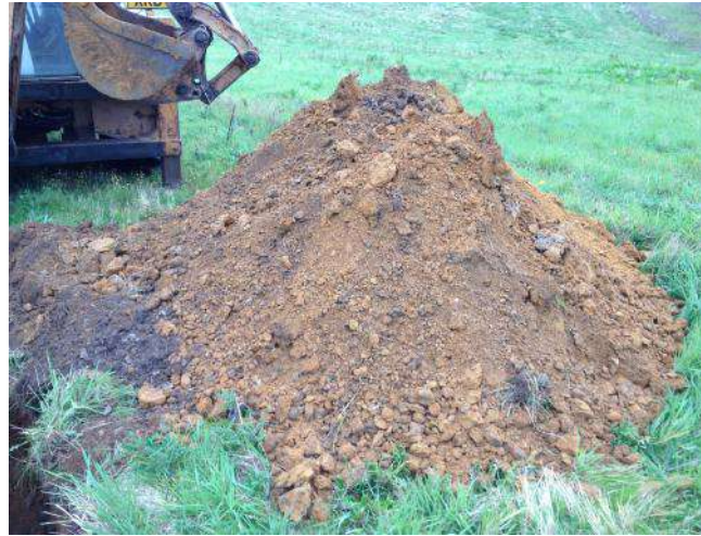
Photo 30: Arisings from trial pit TP13.
