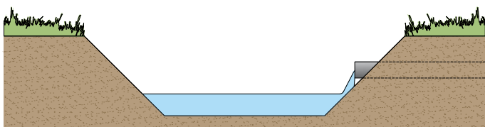
Piped outfall protruding from bank with or without an associated headwall - Consent Required under Section 23 1(b&c)
