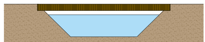
Bridge where soffit level is below the top of bank - Consent Required under Section 23 1(a)
